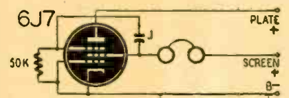
This low-voltage transitron audio oscillator produces a pure sine-wave note at 800 cycles.
